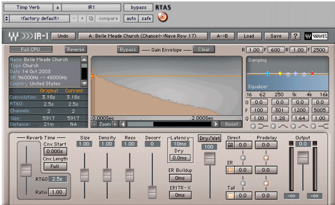
The sampling-type reverb plug-in used for the natural reverb tail. IR-1 reverb by Waves.
